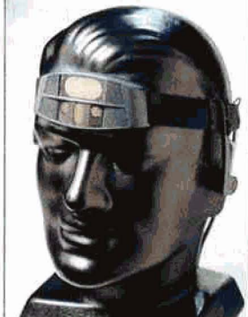
1998: KASPA mimics the sonar capabilities of bats and collects information for blind wearers.
